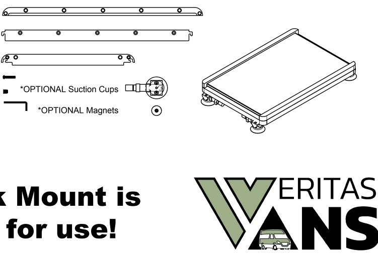
Screw in suction cups or magnets to the inserts on the bottom pieces.
