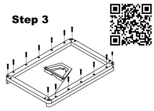
Place the Starlink upside down on a flat surface. Position each top piece on the sides of the Starlink.
